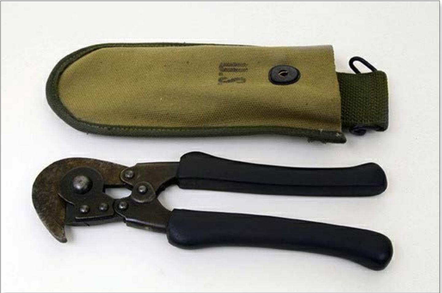
Wire cutters were used to cut through barbed wire and other obstacles.
