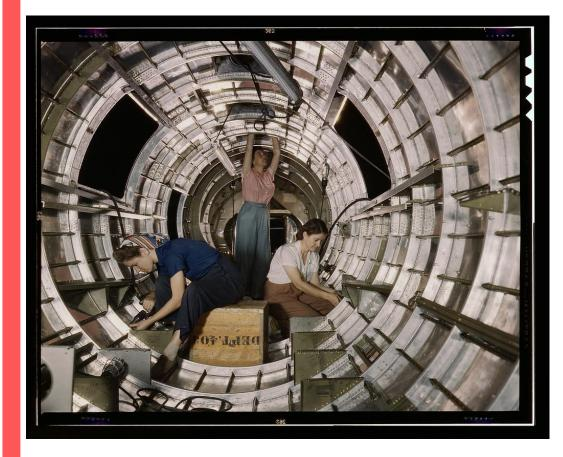
Women workers install fixtures and assemblies to a tail fuselage section of a B-17F bomber at the Douglas Aircraft Company, Long Beach, Calif. Better known as the "Flying Fortress," the B-17F is a later model of the B-17 which distinguished itself in action in the South Pacific, over Germany and elsewhere. It is a long range, high altitude heavy bomber, with a crew of seven to nine men, and with armament sufficient to defend itself on daylight missions
