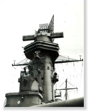
The SG Surface Search RADAR unit on the forward face of the tower on the USS Washington, photographed at the New York Navy Yard on August 18, 1942. U.S. Navy.
