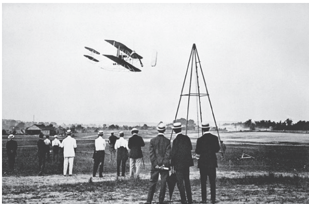
The Wright brothers test fly their aircraft on Fort Myer's parade field. This series of test flights resulted in the Army purchasing its first aircraft. In the first flight, Sept. 9, 1908, Orville Wright kept the plane aloft 71 seconds. National Archives and Records Administration (6641435).
