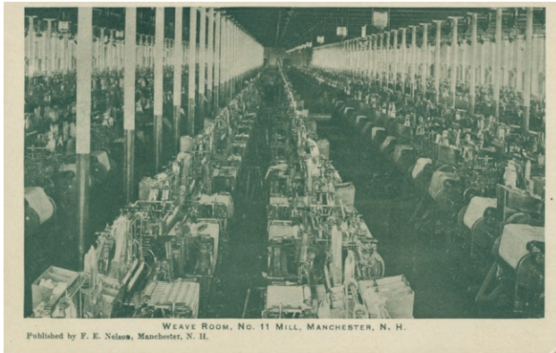
A photo of the weaving room at one of the Amoskeag mills. Here, the looms weave the cotton into cloth, c.1872. F. E. Nelson, New Hampshire Historical Society.
